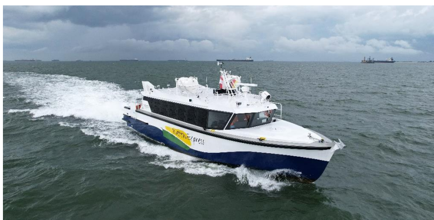
18m passenger ferry with IMO Tier III engines
