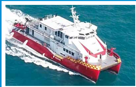
Fast and Furious: 35-knot FiFi-1 Classed Fire Fighting Search-and-Rescue vessel built for the Singapore Civil Defence Force.
